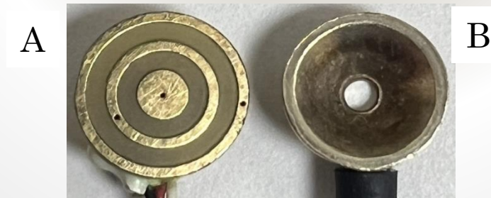
Figure 1. Laboratory sensor equipment includes tripolar concentric ring electrode (A) and conventional disc electrode (B).
