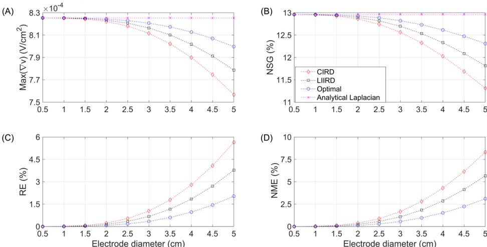
**Figure 6** (top). Maximum Laplacian amplitude (A), normalized spatial gradient (B), and relative (C) and normalized maximum (D) errors of Laplacian estimation computed via FEM modeling for tripolar CREs.
