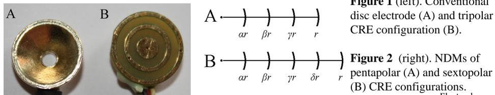
**Figure 1** (left). Conventional disc electrode (A) and tripolar CRE configuration (B).
