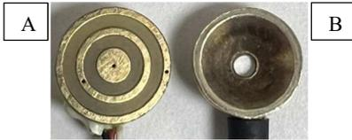
**Fig. 1.** Tripolar concentric ring electrode with dimensions identical to t-Lead from CREmedical (A) and conventional disc electrode (B).
