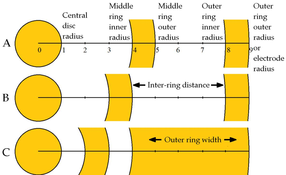
**Figure 2.** Finite dimensions models of three tripolar concentric ring electrode configurations, including: (A) constant inter-ring distances configuration, (B) linearly increasing inter-ring distances configuration, and (C) optimal configuration with respect to the accuracy of the Laplacian estimation.
