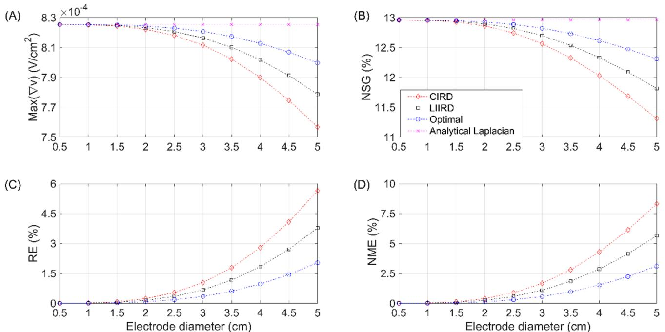
**Figure 4.** Maximum Laplacian amplitude ( $\text{Max}(\nabla v)$ ), normalized spatial gradient (NSG), relative (RE), and normalized maximum errors (NME) computed via the finite element method modeling for tripolar concentric ring electrode diameters ranging from 0.5 cm to 5 cm and a dipole depth of 3 cm.
