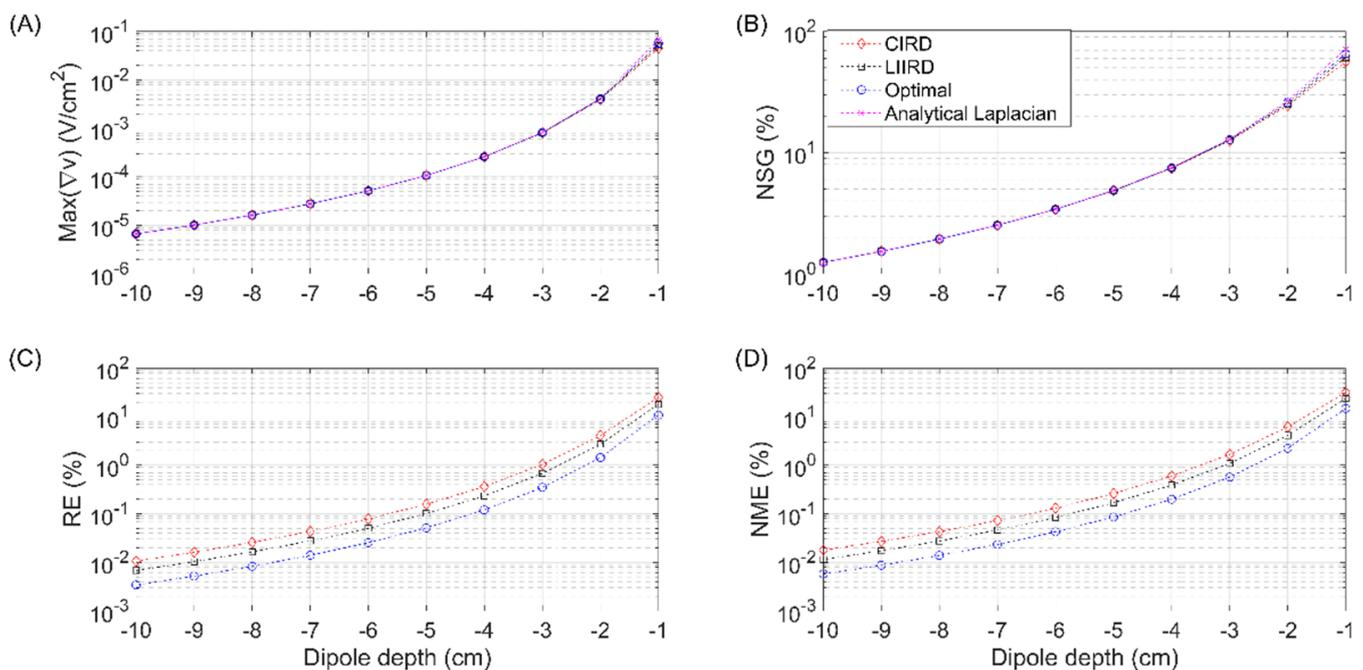
**Figure 5.** Maximum Laplacian amplitude ( $\text{Max}(\nabla v)$ ), normalized spatial gradient (NSG), relative (RE), and normalized maximum errors (NME) computed via the finite element method modeling for a tripolar concentric ring electrode with a diameter equal to 3 cm and dipole depths ranging from 1 to 10 cm.
