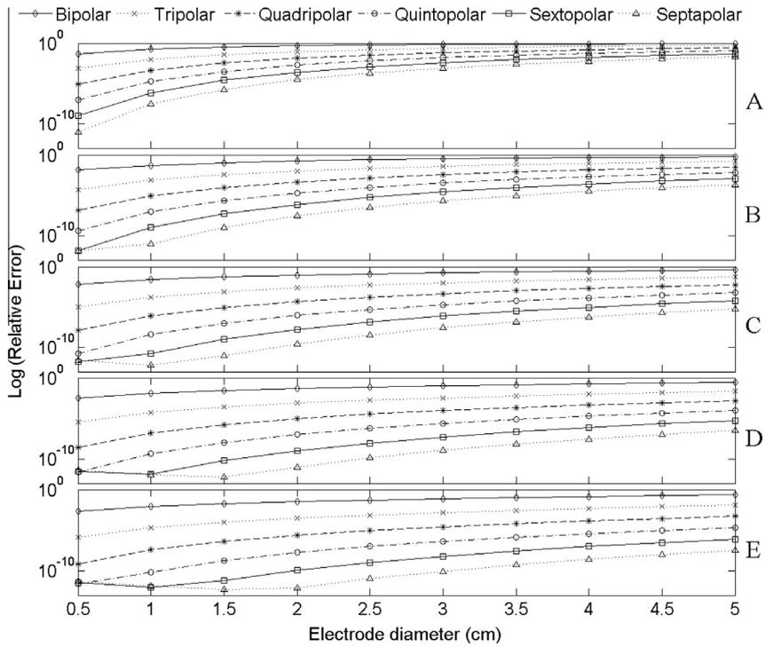
**Fig. 4.** Relative Error of six Laplacian estimates corresponding to the bipolar, tripolar, quadripolar, quintopolar, sextopolar, and septapolar CRE configurations for multipolar CRE diameters ranging from 0.5 cm to 5 cm. Panels A–E correspond to dipole depth ranging from 1 cm to 5 cm respectively.
