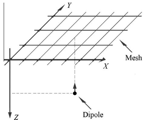
Fig. 3. Schematic of the finite element method computer model with a square mesh of size  $1700 \times 1700$  used to assess and compare the accuracy of Laplacian estimates for multipolar concentric ring electrode configurations ranging from bipolar to septapolar.
