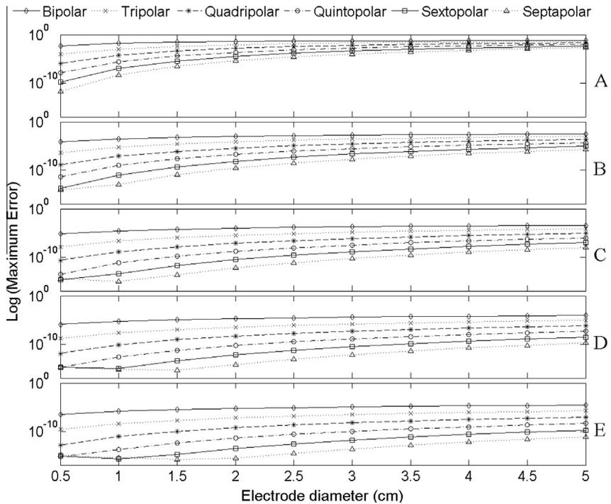
**Fig. 5.** Maximum Error of six Laplacian estimates corresponding to the bipolar, tripolar, quadripolar, quintopolar, sextopolar, and septapolar CRE configurations for multipolar CRE diameters ranging from 0.5 cm to 5 cm. Panels A–E correspond to dipole depth ranging from 1 cm to 5 cm respectively.
