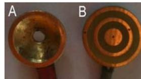
Fig. 1. Conventional disc electrode (A) and tripolar concentric ring electrode (B).
