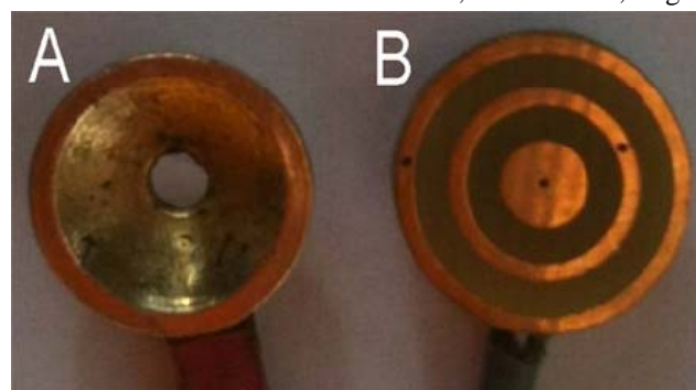
Fig. 1. Conventional disc electrode (A) and tripolar concentric ring electrode (B).
