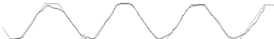
Fig. 7. Result of HEA approximation of the distorted real contour with the theoretical one (number of generations=5, fitness function=15,253).
