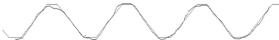
Fig. 8. Result of HEA approximation of the distorted real contour with the theoretical one (number of generations=25, fitness function=8358).
