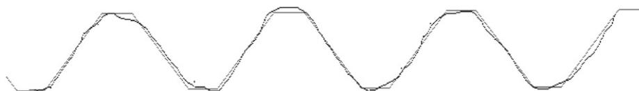
Fig. 9. Result of HEA approximation of the distorted real contour with the theoretical one (number of generations=100, fitness function=5844).
